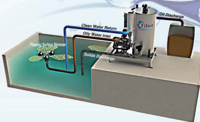
Typical pit or tank installation with a floating oil skimmer.
